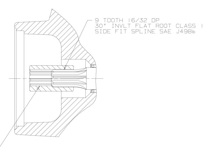
THIS UNIT WILL ACCEPT ANOTHER UNIT WITH AN SAE A MOUNT AND A 9 TOOTH SPLINE 31.8 [1.25] LONG FROM MOUNTING FLANGE ADDITIONAL UNITS DRIVEN BY THIS SPLINE MUST NOT REQUIRE MORE THAN 74.6 N·m [55 16f·f+] TORQUE
